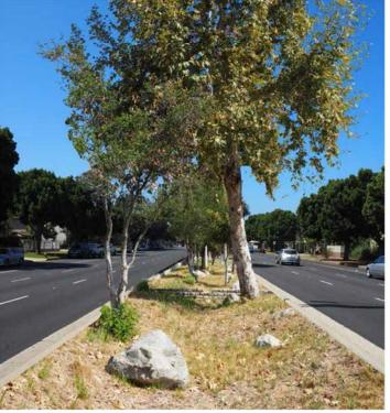
Potential median with stormwater infiltration swale and native planting with irrigation. An existing median infilration treatment on Western Heritage Way in the City of LA can be looked at as an example.
